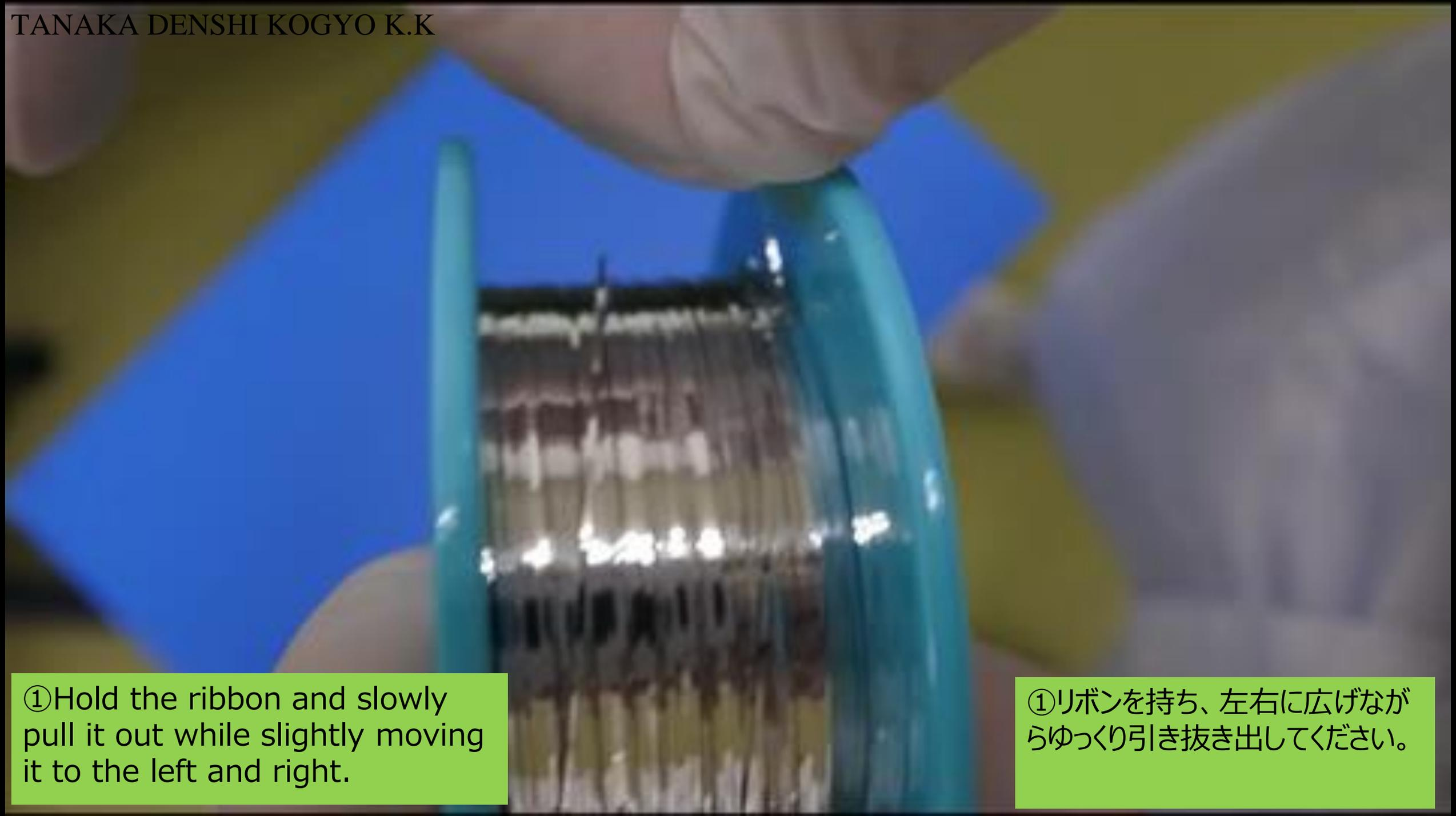
① Hold the ribbon and slowly pull it out while slightly moving it to the left and right.
